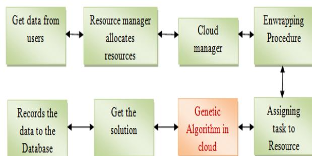
Fig-3 Proposed system of Task scheduling using GA
