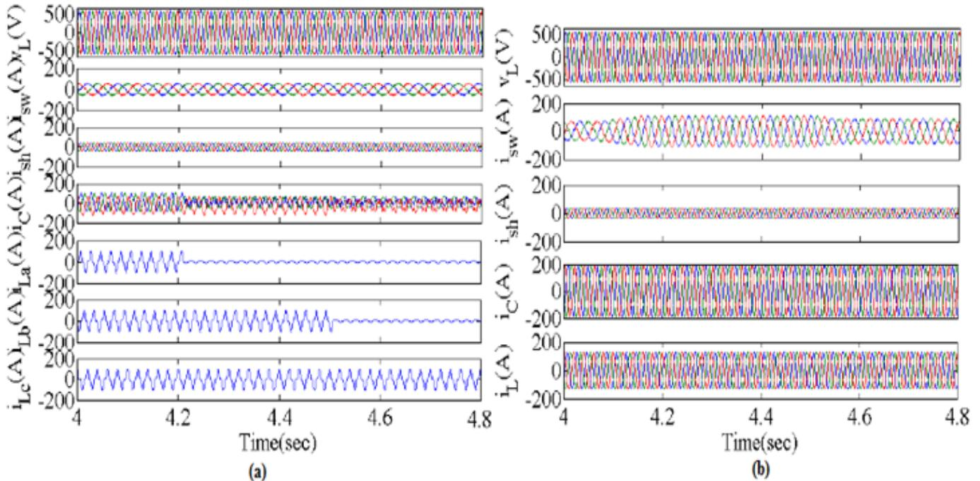
**Fig.1 Performance of the system with (a) non linear load at wind speed of 7 m/s and (b) balanced linear load at variable wind speeds**
