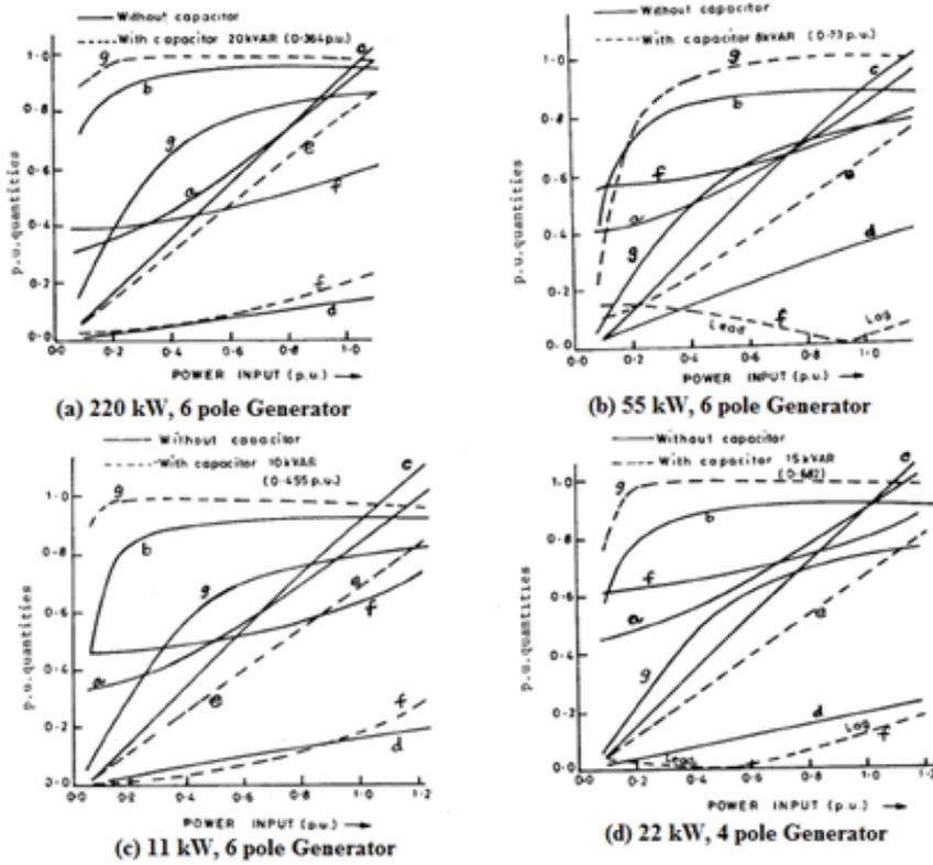
Fig. 3 Characteristics of wind driven IG at varying power input
