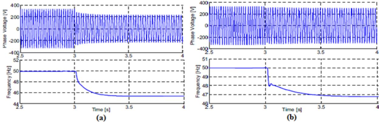
**Fig. 2 Phase voltage and frequency for (a) average load and (b) small load**
