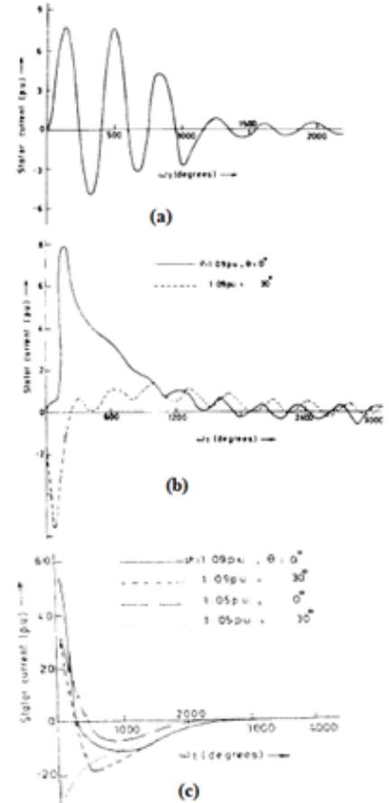
Fig. 4(a) Run-up transient (b) Re-switching transient and (c) Short circuit transient
