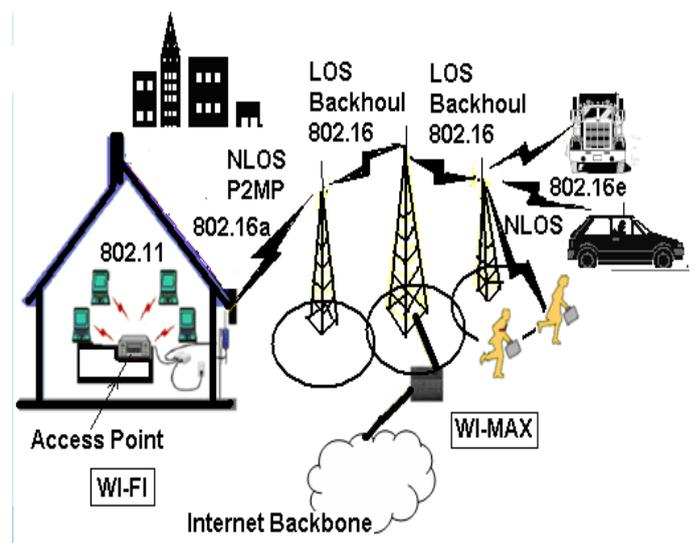
Figure: 1 Fixed and Mobile Wimax
