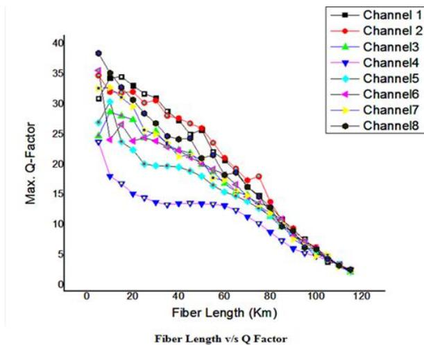
Fig. 2 Effect of fiber length on Q-Factor (with EDFA)
