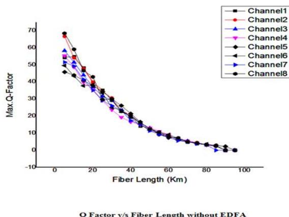
Fig. 3 Effect of fiber length on Q-Factor (without EDFA)
