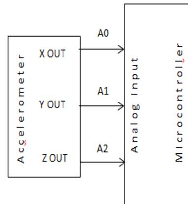
Figure 3:- Accelerometer outputs to microcontroller
