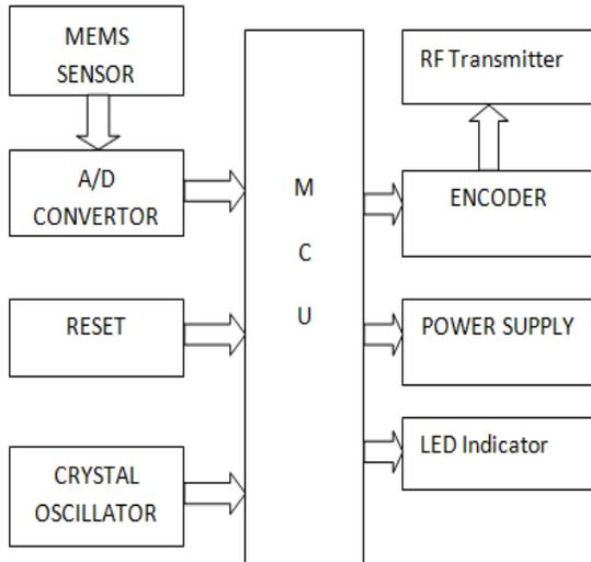
Figure:- 2.1:- Transmitter Block
