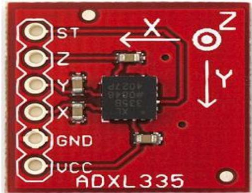
Figure 1.2. ADXL 335 Accelerometer
