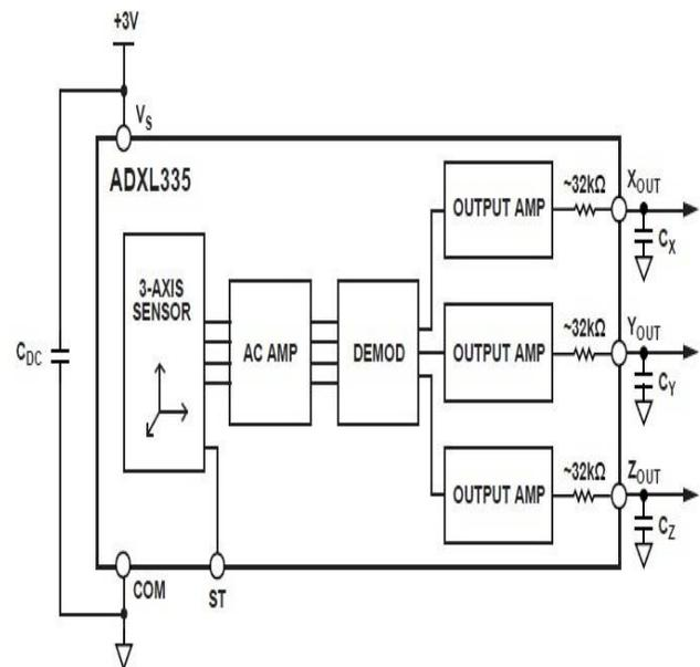
Figure 1.1:- Block diagram of ADXL 335
