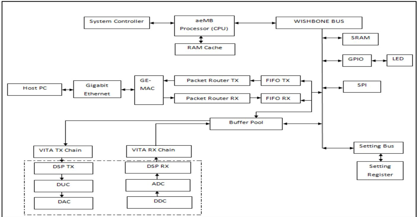
Fig.2 Internal Components of USRP FPGA
