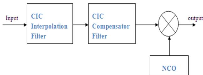
Fig:5 Block diagram of DUC
