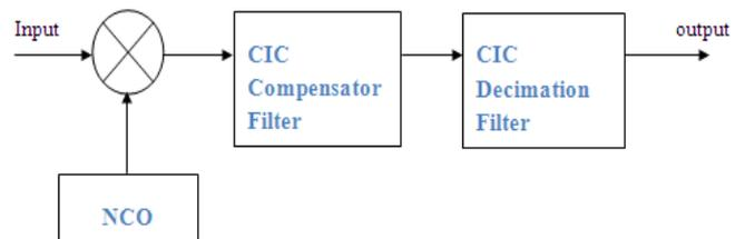
Fig:6 block diagram of DDC
