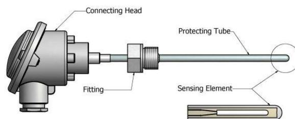
Fig. 3. Resistance Temperature Detector
