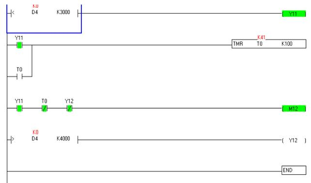
Fig. 8. Ladder Diagram For Water Level Control
