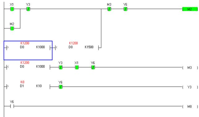
Fig. 7. Ladder Diagram for Temperature & Pressure Condition
