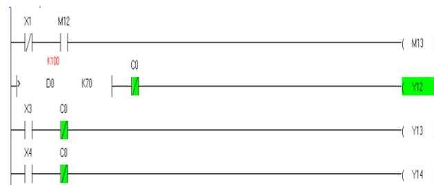
Fig. 4. Ladder diagram for high temperature detection.
