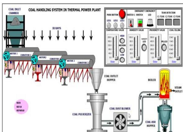
Fig. 6. SCADA design for Coal handling system in thermal power plant.
