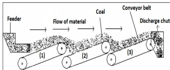
Fig.1. Interlocking Protection in belt Conveyor.
