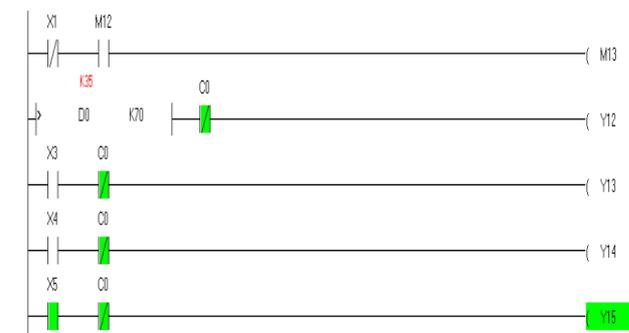
Fig. 5. Ladder diagram for conveyor belt tear up detection.
