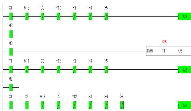
Fig. 2. Ladder diagram for startup sequence of the belt conveyor.
