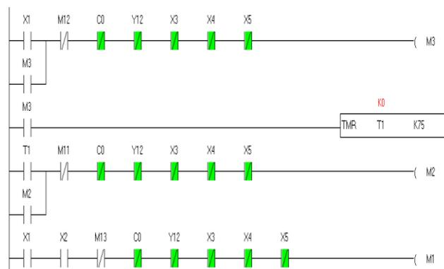
Fig. 3. Ladder diagram for stopping sequence of the belt conveyor.
