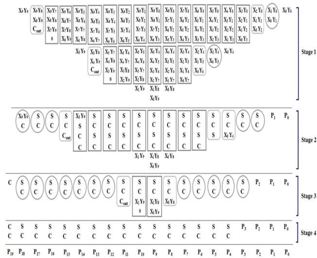
Fig. 6: 10x10 Wallace Tree Multiplier based on 4-2 Compressors
