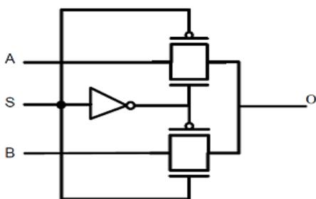
Fig. 2: MUX using transmission gates
