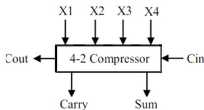
Fig. 3: Block diagram of 4-2 Compressor
