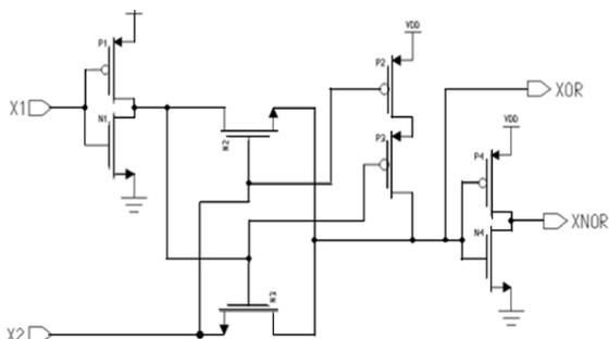
Fig. 1: Circuit diagram of XOR-XNOR
