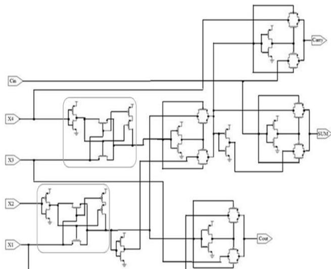
Fig. 4: Transistor model of 4-2 Compressor
