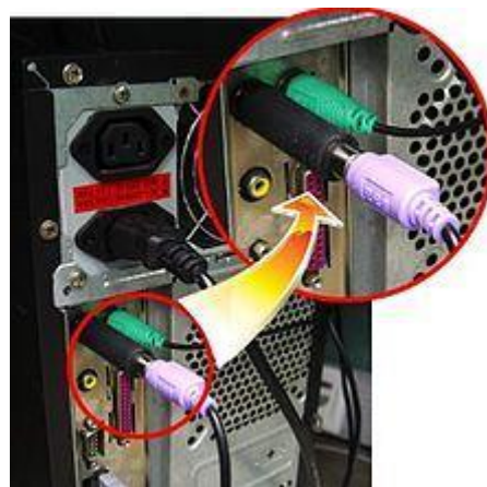
Fig 2: A connected hardware-based keylogger
