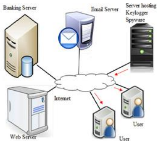
Fig 3: Keylogger Spyware attack on User' s system
