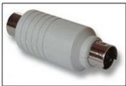
Fig 1: A hardware-based keylogger.
