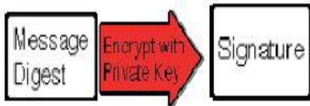
Fig.3 Encryption of message digest signature
