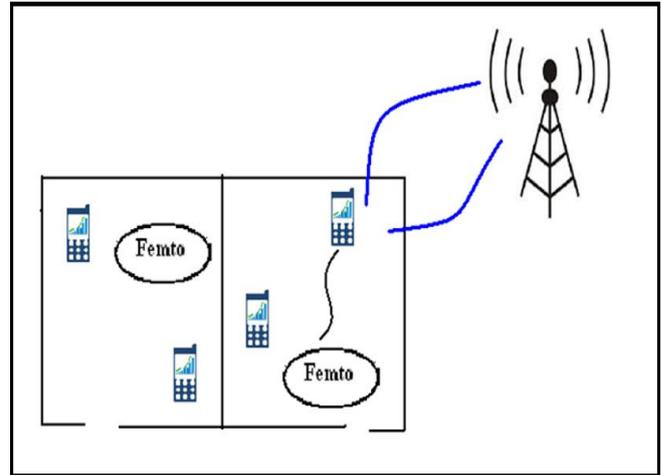
Figure 5. Cross-Tier Interference for the Downlink and Uplink
