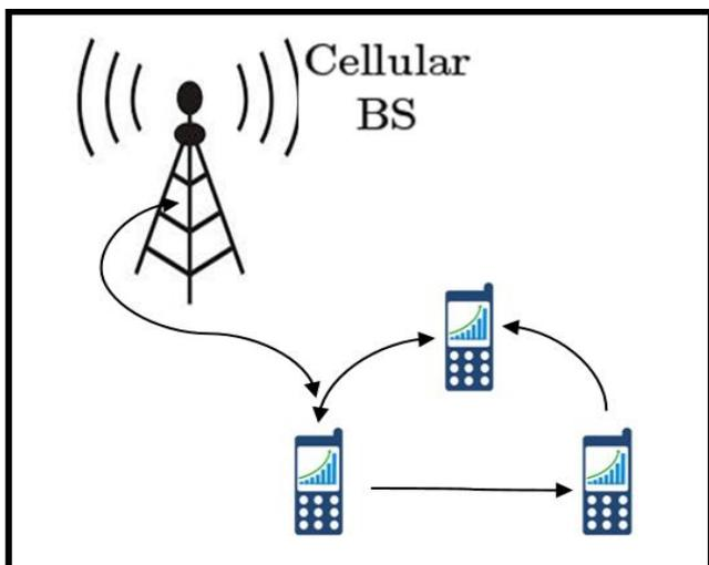
Figure 3. Mobile Data Offloading Via Disruption Tolerant Networking
