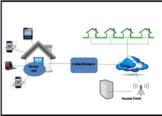
Figure 4. Mobile Data Offloading Via Femtocells.
