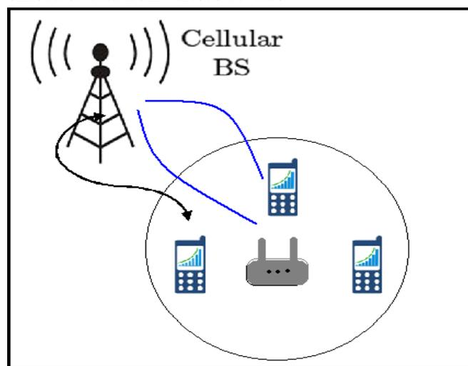
Figure 2. Mobile data offloading using LTE small cells.
