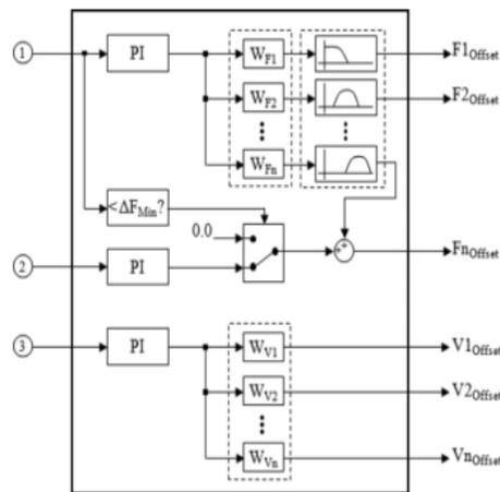
Fig. 3 Microgrid Central Controller
