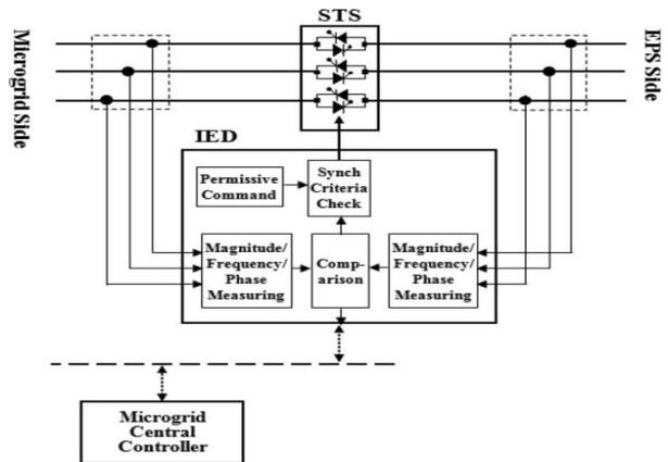
Fig. 2 Block diagram of IED
