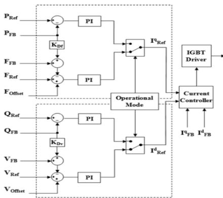
Fig.4 Control structure of BESS inverter.
