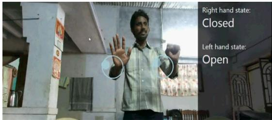
Fig 5. Hand point position detection and basic gesture recognition
