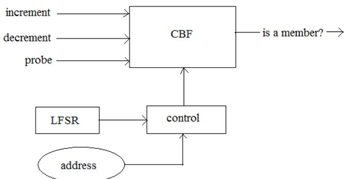
Fig.4. Block diagram of Counting Bloom Filter
