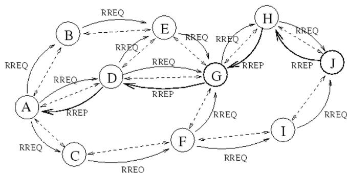
Fig. 2 Route discovery procedure in MANET using DSR
