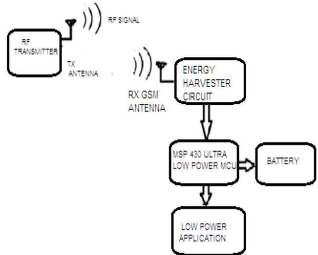
Fig.2. Block diagram of Energy Harvesting System.
