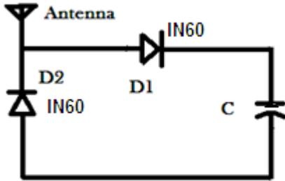
Fig .3. Basic Harvester Circuit
