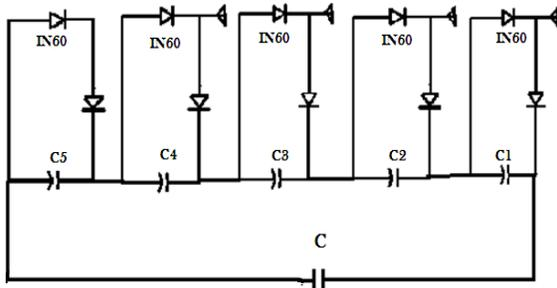
Fig.4. Multistage energy harvester circuit
