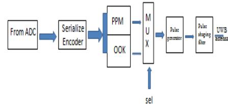
Figure 4. Block Diagram of Wideband Telemetry system
