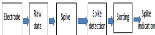
Figure 6. Block Diagram of Sorted Method
