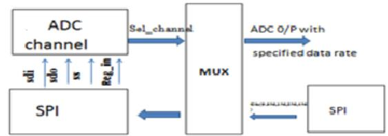
Figure 3. Block Diagram for Selection of a channel
