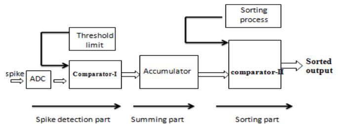
Figure 7. Internal Architecture of Sorted Method
