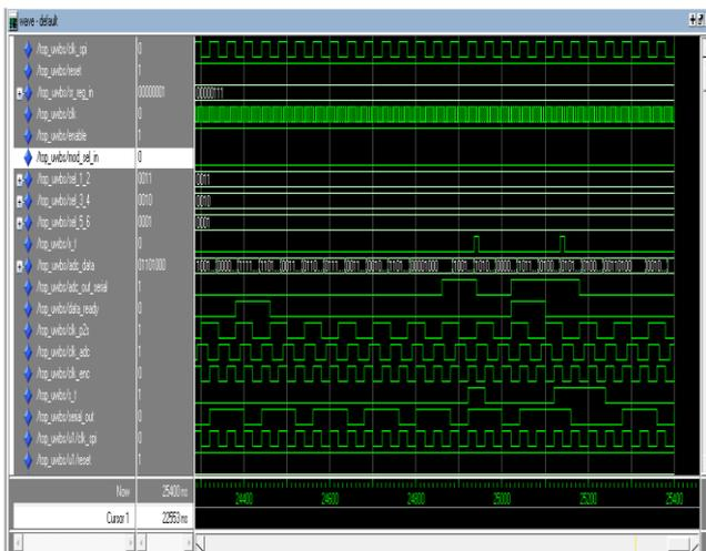
**Figure 9(a).** Simulation Result for Pulse Generation of OOK UWB Signal
