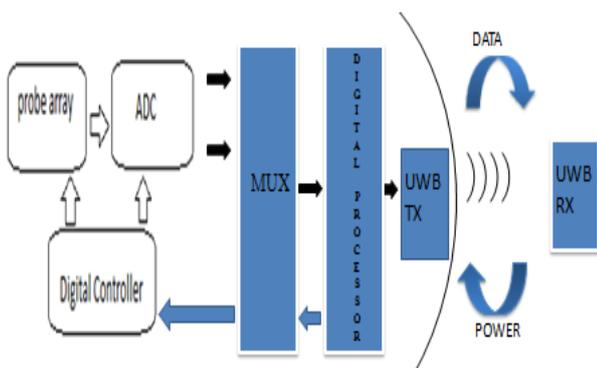
Figure 2. Block Diagram of the Sequentially Turn-On-Method
