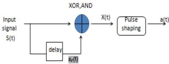
Figure 5. IR-UWB Pulse Generation
