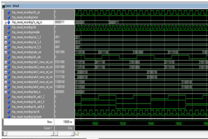
**Figure 8.** Simulation Result for the Selection of a Channel with Specified Clock Rate Based on Sequential Turn-On Method
