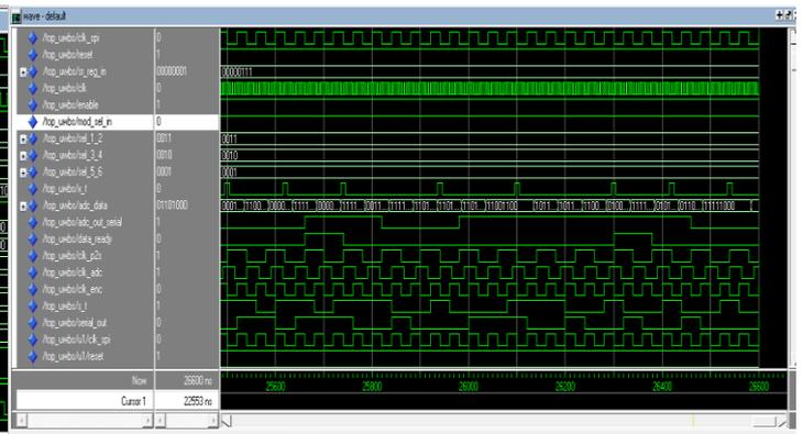
**Figure 9(b).** Simulation Result for Pulse Generation of PPM UWB Signal
