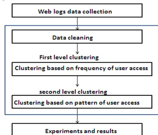
Figure 2 - Two level clustering proces
