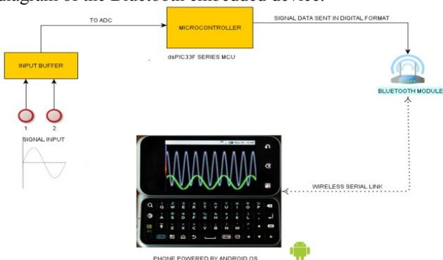
Figure 1 : Functional Block diagram of Wireless Graphical probe system.
