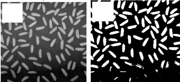
Fig 2 ( a ) purposely adds a white object to (a) increase its distance ratio . Result is given in Fig 2(b) as the weak objects at the bottom are failed to be segmented.
