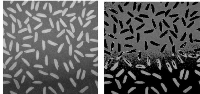
Fig 5(a). Normalized input image, Fig 5(b). Image with TBD region identified.
