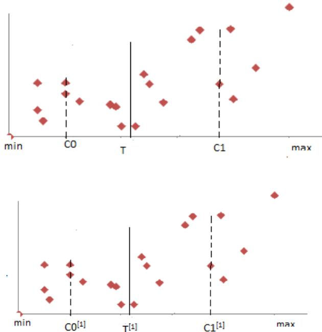
Fig 4(a) otsu method separates image into three regions in the first iteration. Fig 4(b) shows the application of otsu segmentation in the TBD region.
