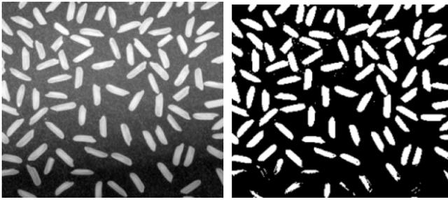
Fig 1 (a): shows the test image, Fig 1(b) :shows the result of standard otsu method.
