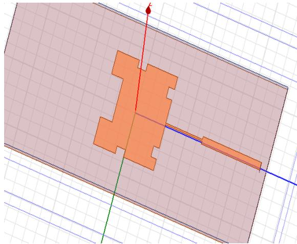
Fig 2: geometry of microstrip patch antenna in U-shape
