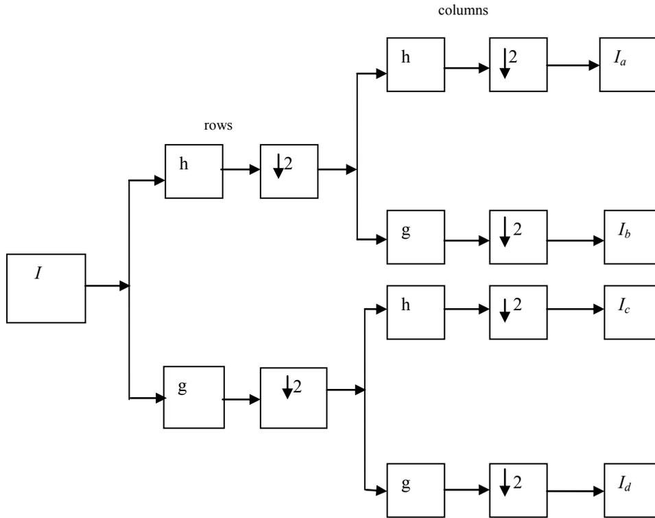
Fig 2. Structure of 2-D DWT
