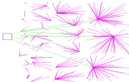
Figure 1. Multihop Routing of 400 nodes in WSN
