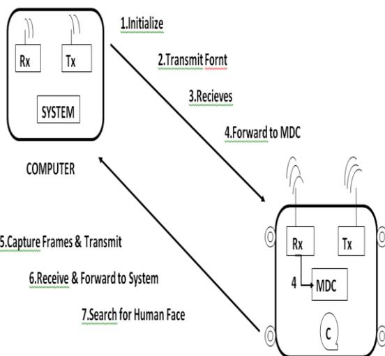
Fig 1 : Working of Robot & Computer
