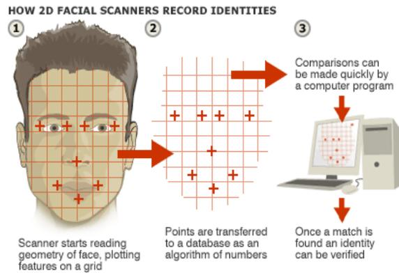
Fig: 2 Face Identification Using HAAR algorithm & System Verification
