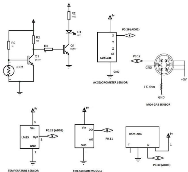
Fig 3 Sensors in Sensor Network
