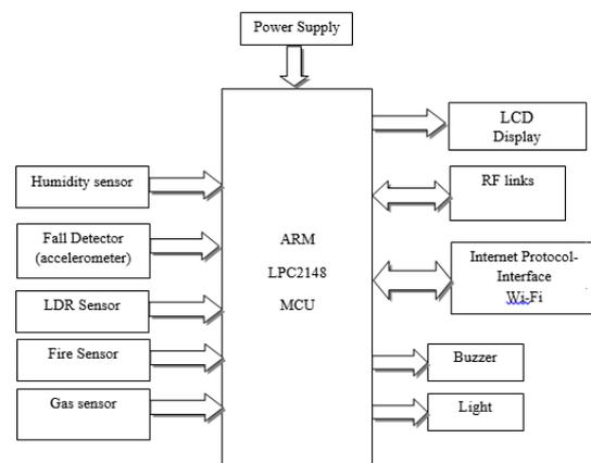
**Fig 1 Interfacing Block Representation of Wearable Device.**
