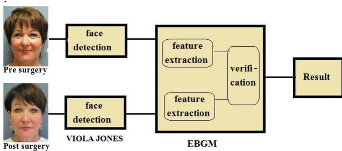
Fig.3 Block diagram illustrating different stage of proposed algorithm
