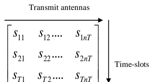
**Fig 1: Representation of Space-Time Block Codes (STBC)**
