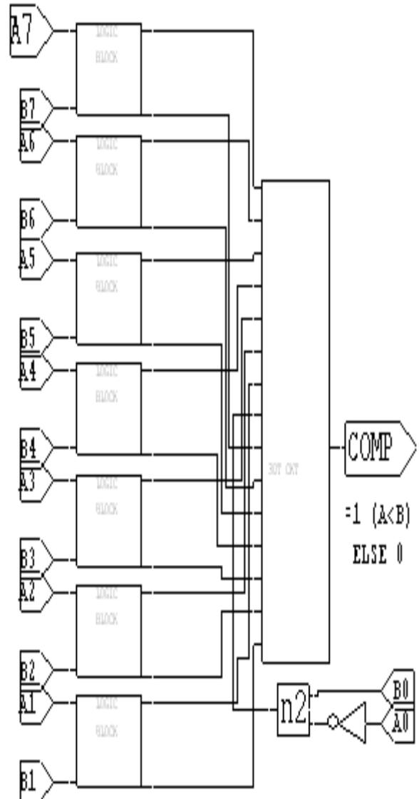
Fig. 3 Schematic of 106 transistor Comparator cell
