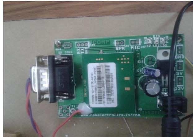
**Fig.4 GSM Board**
