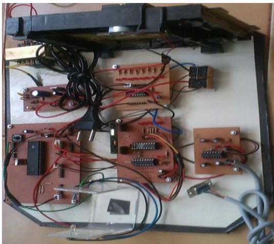
Fig.6 Receiver Section
