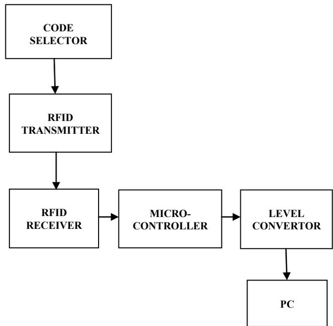
Fig.2 Block diagram for Automatic payment module
