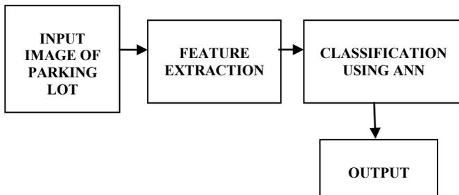
Fig.1 Block diagram for Vehicle Counting Module
