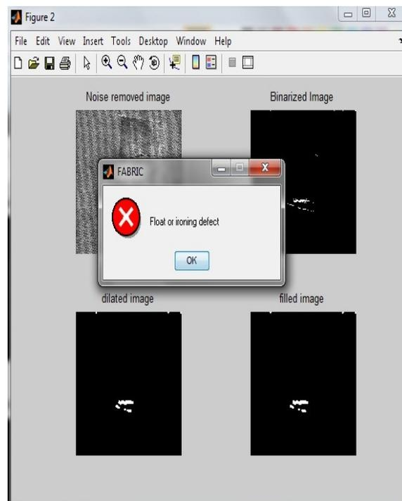
Fig. 4. Images of fabrics at different process of defect detection, the corresponding binary detection results and classification of defect by ANN classifier.
