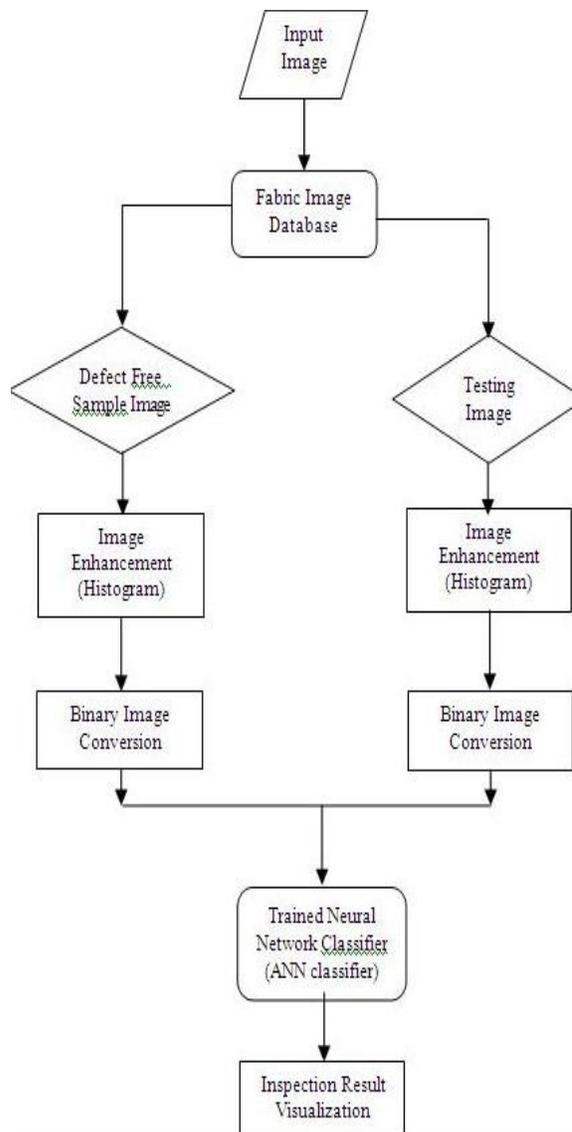
Fig. 3. The flowchart of the Image Decomposition method for pattern fabric inspection.
