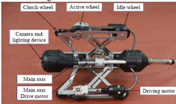
Fig. 1. The developed robot.
