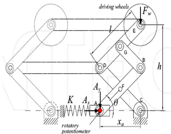
Fig 4. Wheeled leg mechanism of MRINSPECT III
