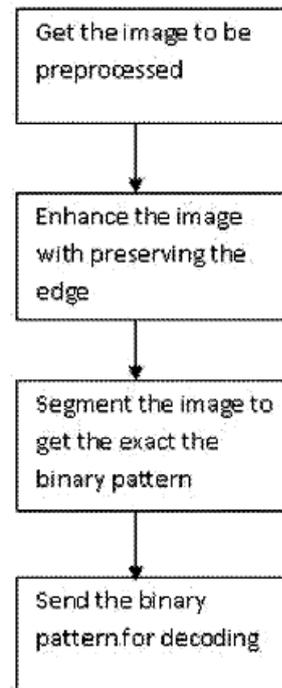
Fig. 5 The preprocessing steps to be applied in the decoding process.
