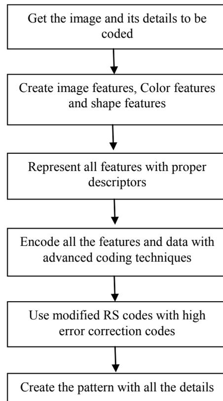
Fig. 2 The flow diagram for the encoding process according to one embodiment of the method of the paper.
