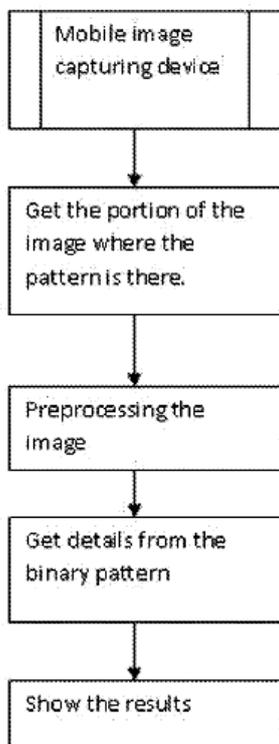
Fig. 4 The flow of the overall decoding process.
