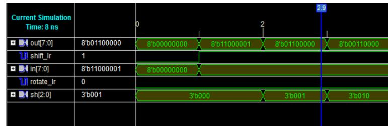
**Simulation waveform of 8-bit Barrel Shifter (right shift)**
