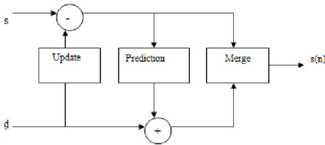
Fig.4.Inverse Lifting Scheme
