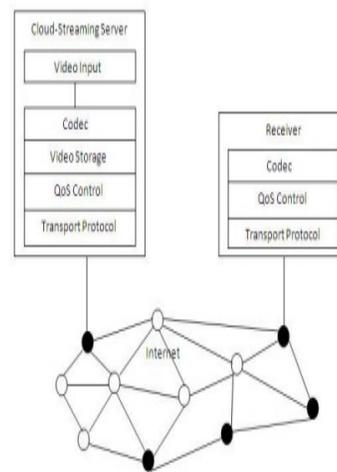
**Fig.2: Video Streaming Architecture**
