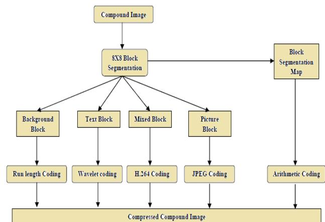
Fig.1 Block Based Compression
