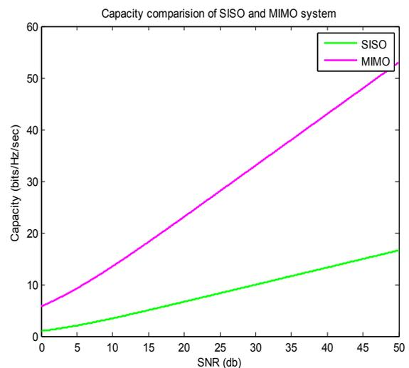
Fig. 7 Capacity comparison of SISO and MIMO system
