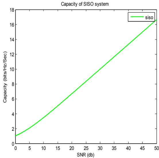
Fig. 6 (a) Capacity of SISO system
