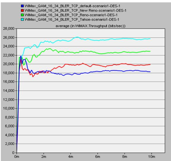
Fig. 8 QAM 16\_34 BLER throughput
