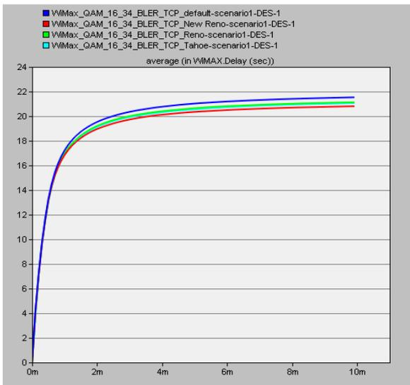
Fig. 4 Average QAM 16\_34 BLER delay
