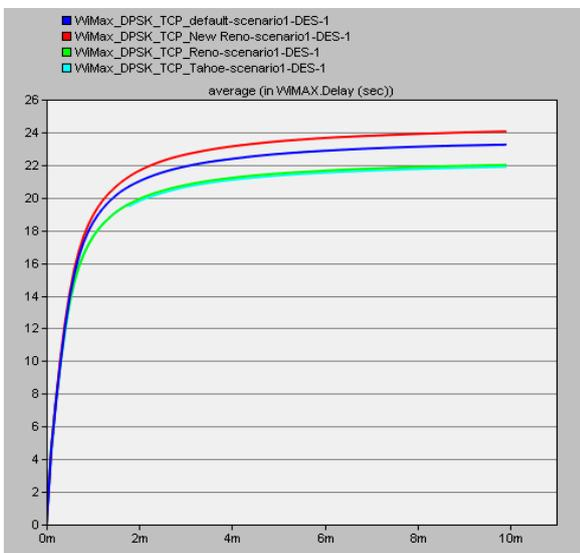
Fig. 3 Average DPSK delay
