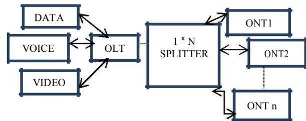
Fig.1 General Schematic of PON Architecture
