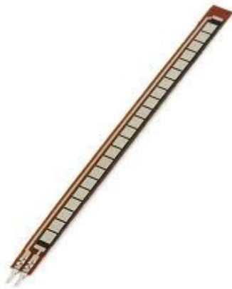
Fig 3. Flex Sensor Strip.
