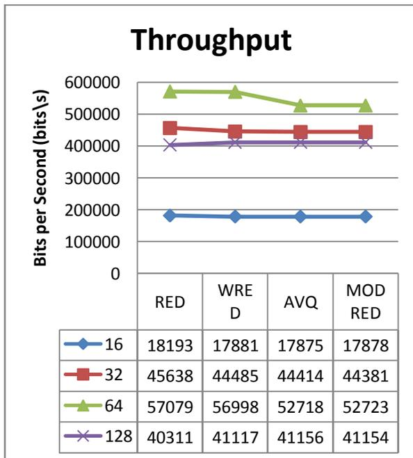
The RED, WRED, AVQ & Mod RED AQMs were tested under different traffic loads, with Strict Priority by varying the number of Nodes in terms of 16,32,64,128 .
