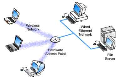
computers. It can connect or bridge the wireless LAN to a wired LAN, allowing wireless computer access to LAN resources, such as file servers or existing Internet Connectivity. (compnetworking.about.com)
