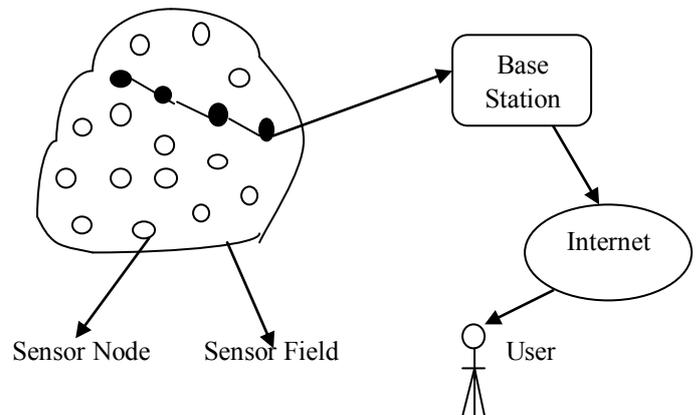
Fig. 1 A Typical Wireless Sensor Network
