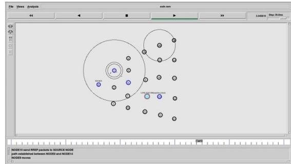
Fig 2: Link failure due to mobility
