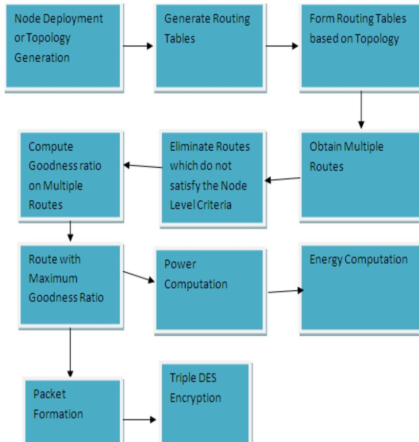
Fig 1: Architecture of the proposed system
