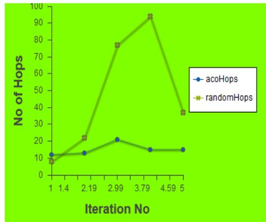
Fig 7: Comparison between Ant Colony Optimization and Random Routing with respect to Hops
