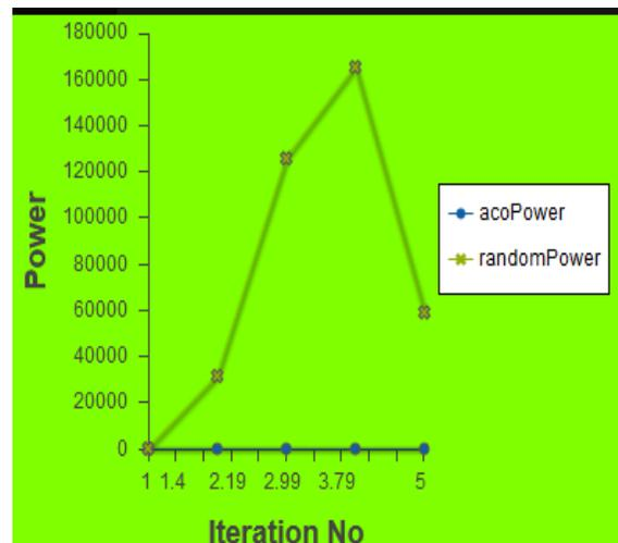
Fig 4: Comparison between Ant Colony Optimization and Random Routing with respect to Power
