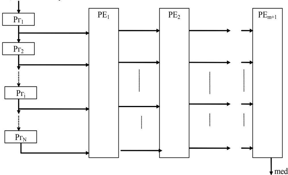
Figure 6. Scheme of median filter based on bitwise comparison
