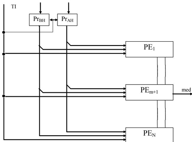
Figure 1. Algorithmic scheme of the one-dimensional median filtering device, which based on the insertion sort method
