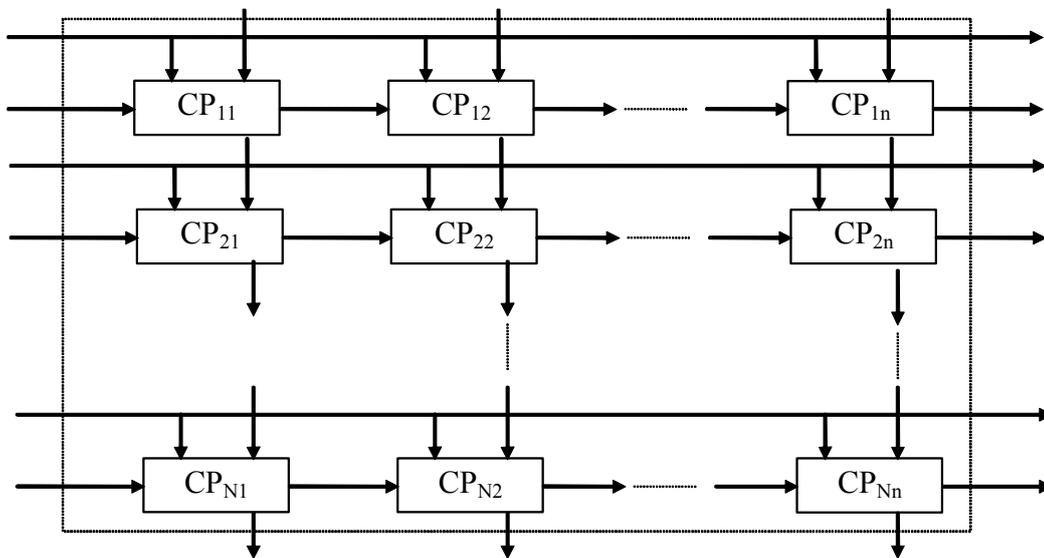
Figure 7. Scheme for PE of median filter based on bitwise comparison
