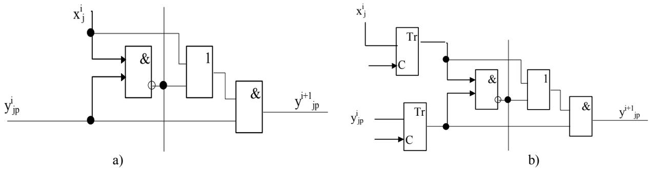
Figure 8. Cells comparison scheme: a) single-cycle unit; b) conveyor device
