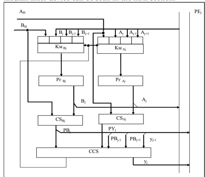
Figure 2. Scheme of the processor element of median filtering device, which based on the insertion sort method
