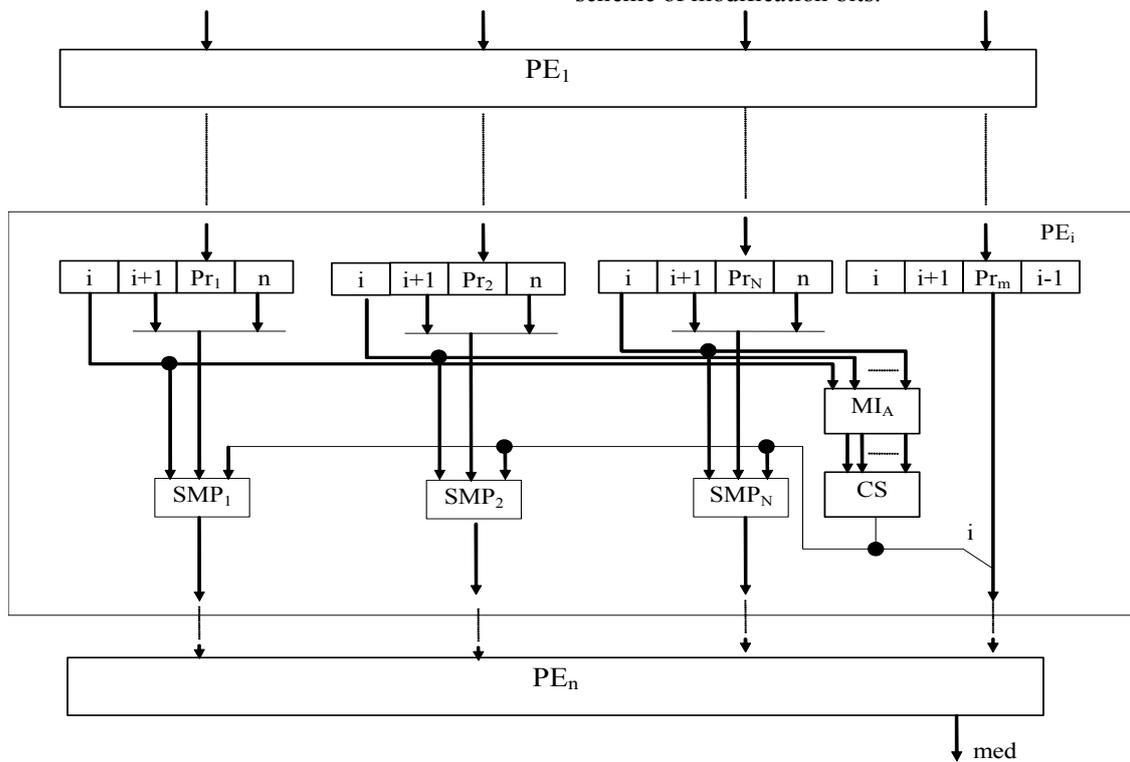
Figure 5. Structure of median filter with consistent calculation of median bits
