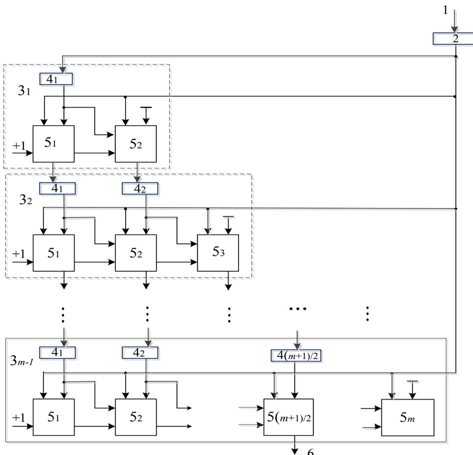
**Figure 3. Scheme of the median filtering device with the filter window of size m**
