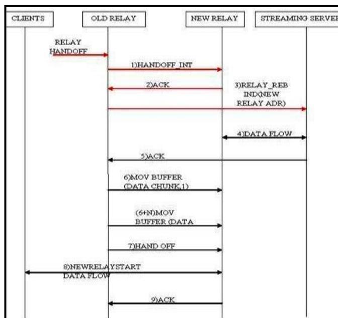
Fig.1 Hand-off management process for spectrum aware PSNR.
