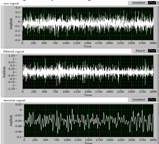
Fig. 3 Raw Surface Electromyogram signals after Band pass filter and DWT denoising
