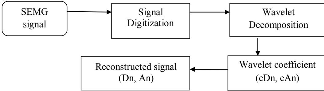
Fig. 1 Block diagram for wavelet analysis of surface Electromyogram signal
