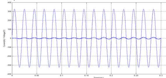
Figure.14 Source voltage and current of phase-a for p.f verification using modified Icos $\phi$  controller.
