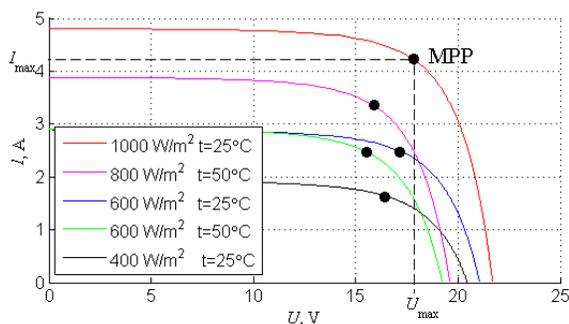
Figure. 2. MPP at different SEF and temperatures.
