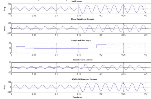
Fig.12. Modified  $I_{cos\phi}$  controller performance comprising of load current, phase shifted load current, sample and hold output, desired source
