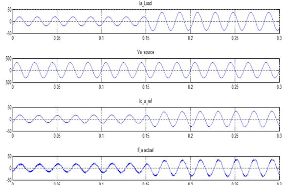
Figure.13. Modified IRPT controller output comprising of load current, source voltage, reference and actual currents
