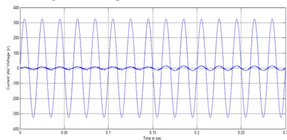
Figure.15. Source voltage and current of phase –a for p.f verification using modified IRPT controller.
