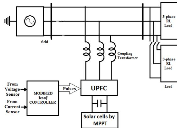
Figure.1 Schematic of the three phase grid system with the UPFC Interface for renewable energy source
