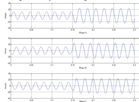
Figure.6. Three phase load currents of RL linear Load
