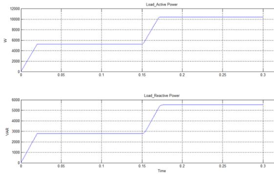
Figure.9. Active and Reactive power of dynamic linear loads.
