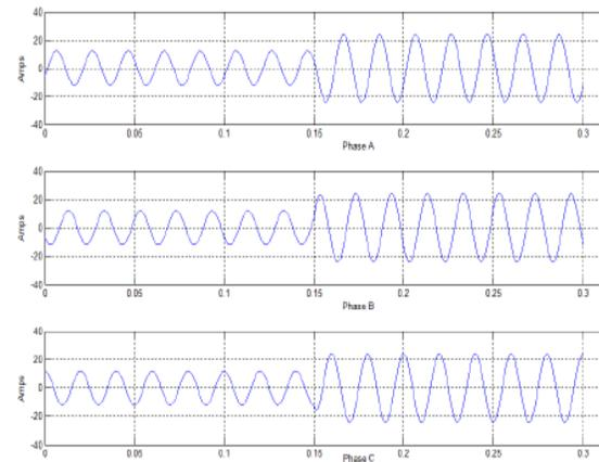
Figure.4. Three phase currents of source (grid) side
