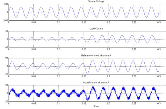
Figure.11. Source voltage, load current, actual current and reference current
