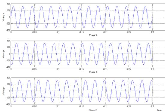
Figure.5. Three phase load voltages of RL linear Load
