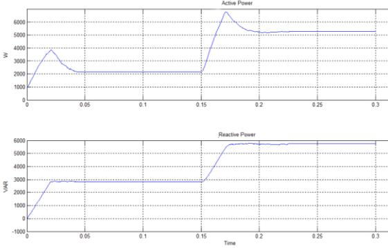
Figure.8. Active and Reactive power of UPFC unit at PCC
